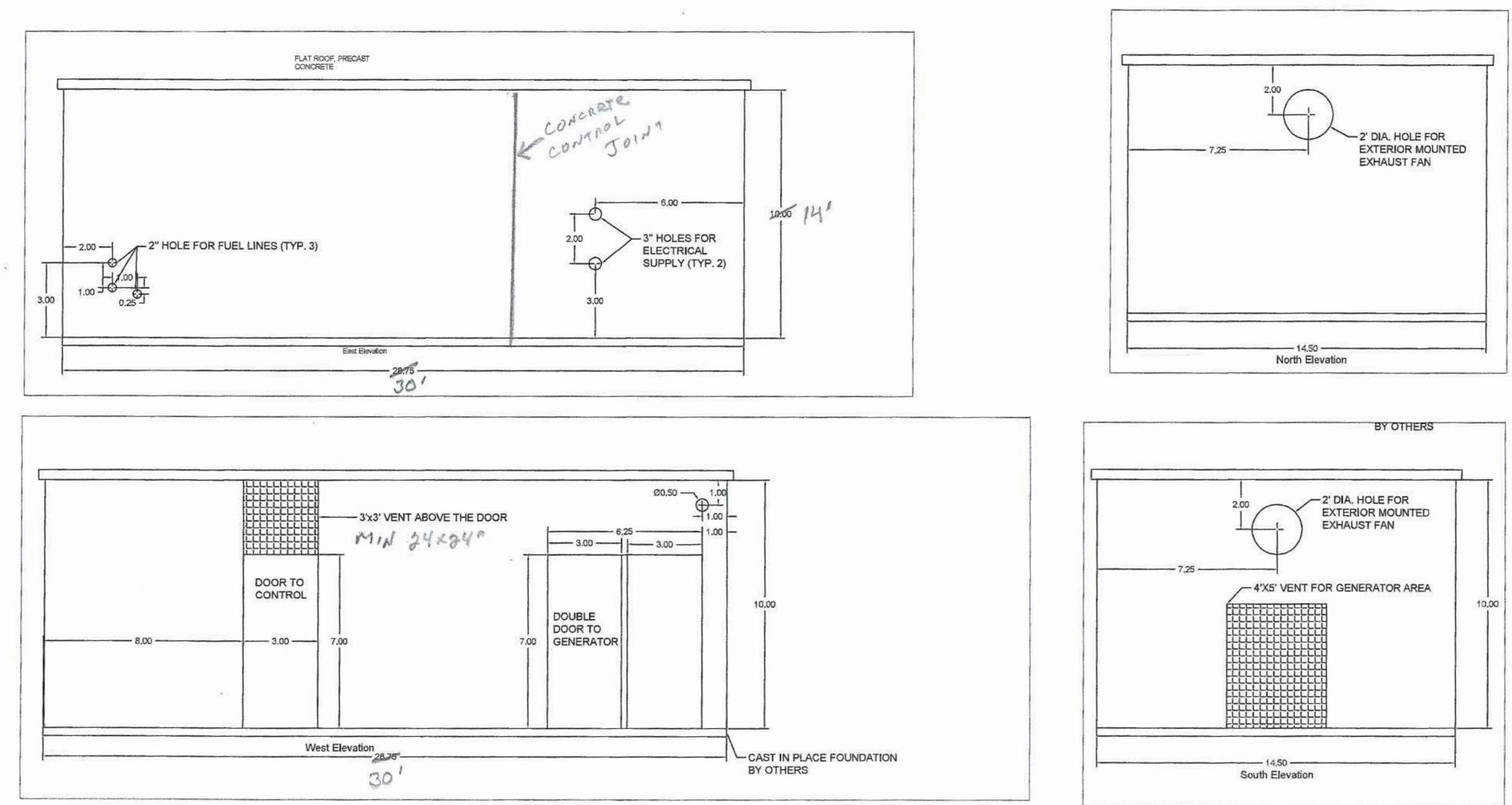
**Preliminary Elevations** Final Drawings to be prepared by Contractors
